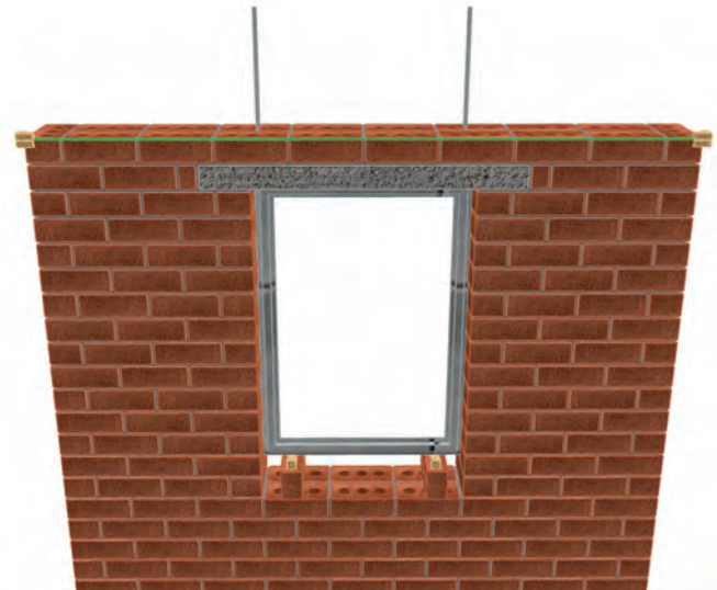
12.16 - Completed project showing built-in pre-cast lintel and roof wire ties.
