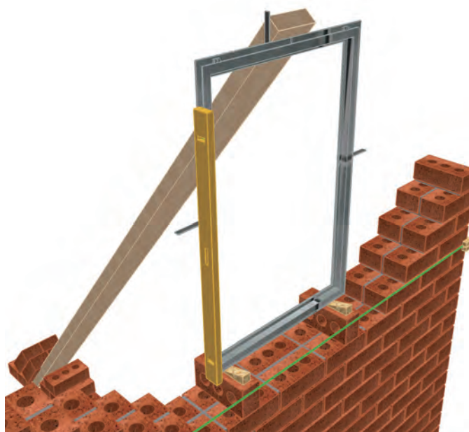
12.8 - Set the frame plumb (level in front) by adjusting the support.
