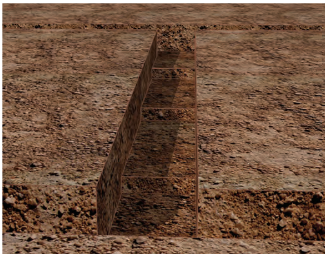
5.13 - Foundation trenches should be dug to a depth of not less than 400mm below the surface all round, following the contours of the ground. The width of the trench is usually twice the thickness of the wall plus 150mm, with a minimum width of 450mm for internal walls. The figure shows how the sides of the trench must be trimmed neatly and square.
