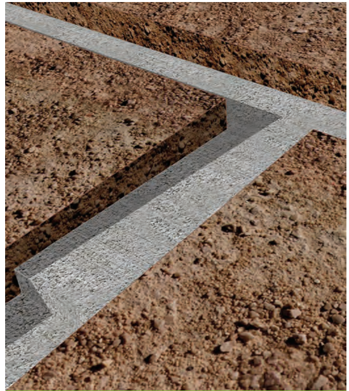
5.19 - Showing completed foundations with steps.
