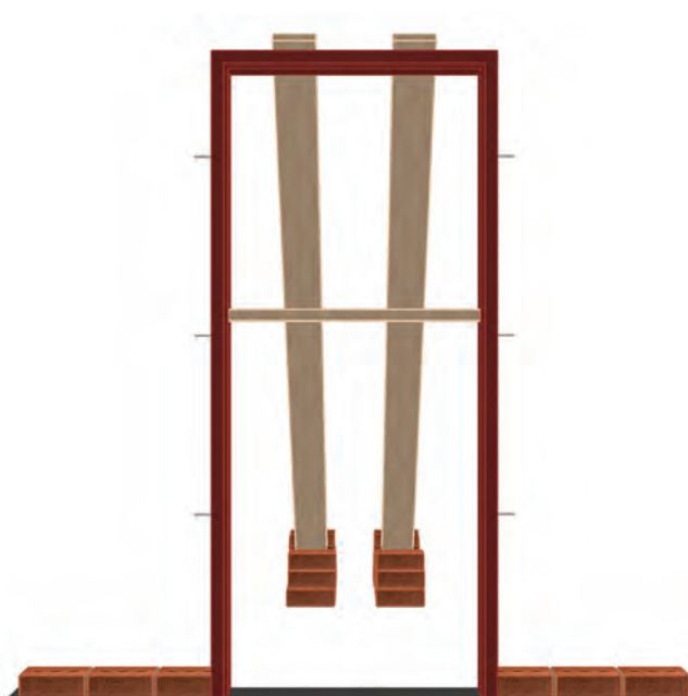
12.21 - Front view of the door frame. NOTE: The lugs and the centre strut (dwang) that is installed to prevent the frame from bulging in during building-in operations.
