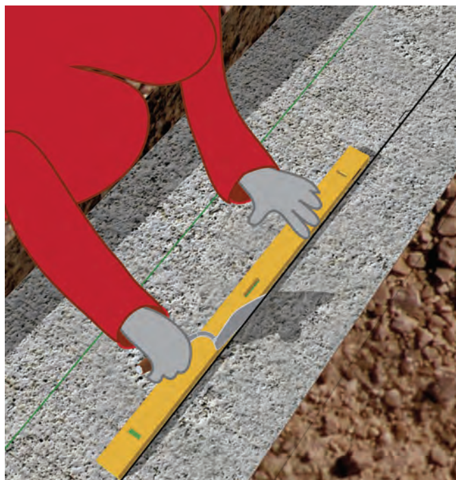
11.11 - After a second line is transferred down a little further along, the lines are joined using a level or straight edge.
