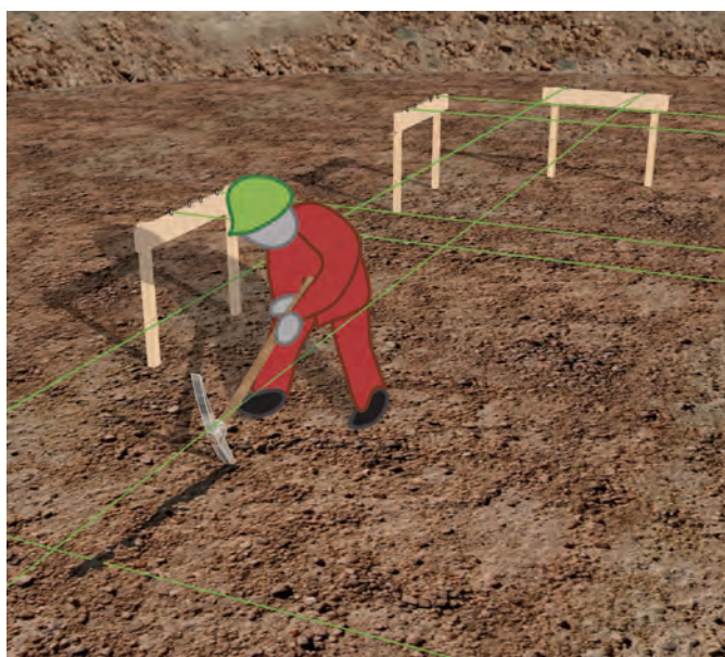
5.11 - The foundation measurements may be transferred to the ground by using a pick as shown
