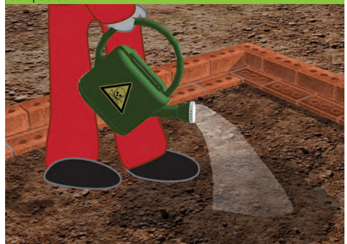
8.5 - Final layer is fully compacted. This layer needs to be poisoned by a specialist contractor. This prevents any infestations below the surface bed.
