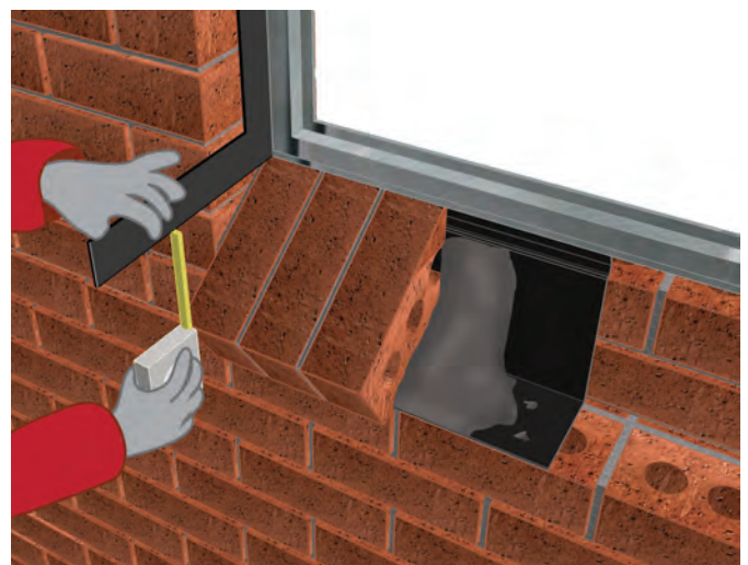
12.18 - Brick-an-edge external sill. The slope of the sill is measured to ensure an equal slope on all the external sills of a particular building. NOTE: The placing of the undersill D. P. C.
