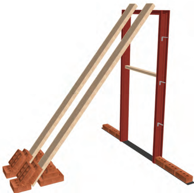
12.20 - Doorframe set upright in position on top of the D. P. C. As with window frames the door frame is secured in position with temporary supports.
