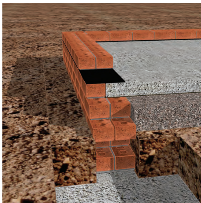
11.18 - Showing D.P.C. for solid superstructure wall construction.
