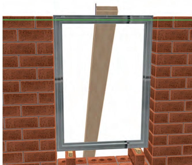
12.10 - The built in window frame projects above the brickwork by a joint thickness.
